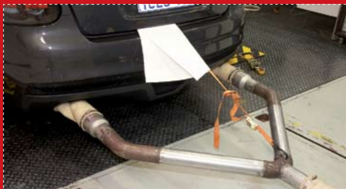
More than just stuffing a sensor up the exhaust pipe, ADR 79/01 requires a sealed exhaust system, and the total waste product is thoroughly analysed
