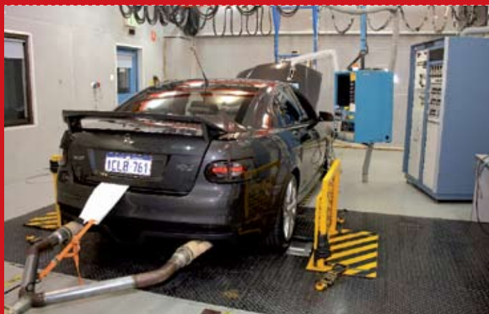
Orbital uses an MRW electrical inertia-simulation dyno from the UK. Although not a particularly common name in our world of dyno shootouts, it is an industry-standard device for emissions testing. It uses a 48in single roller connected to a 200kW DC motor for load absorption and control
