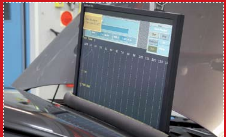
Look closely and you will see the crosshairs. Chris has to keep the "Target" on a set course using the accelerator and gears. No deviation from the course is allowed
