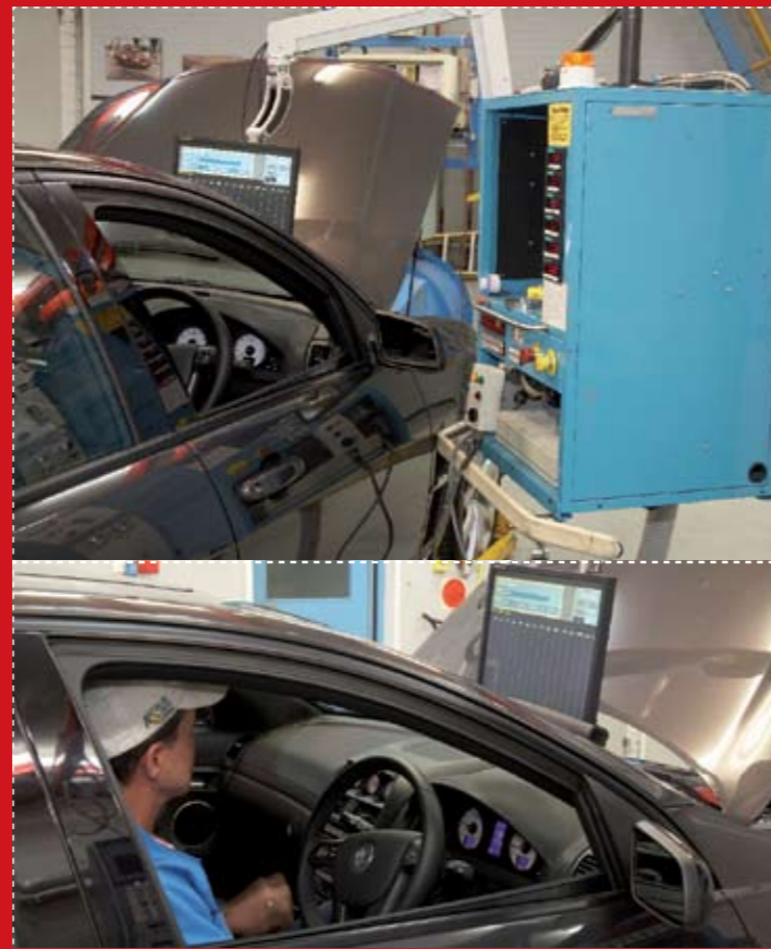
Using the gears and accelerator, the operator must follow a set course that the computer screen determines
