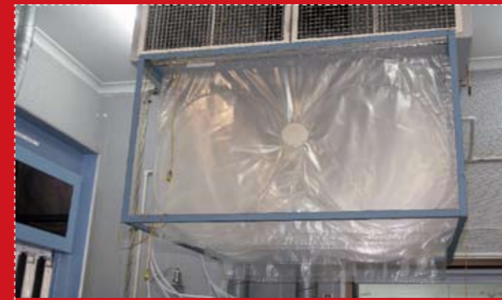
All of the nasty stuff is stored in these bags in diluted form and the computer then calculates the parts per million
